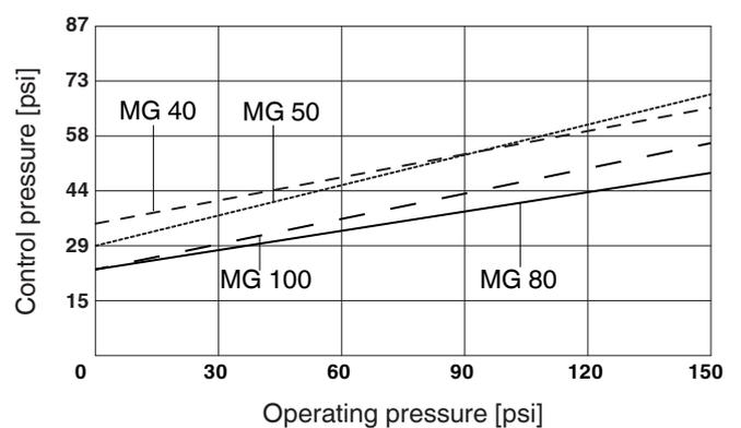
The control pressure depending on the prevailing operating pressure, as shown in the diagram, is intended as a guide for operating the system with low wear on the diaphragm.
