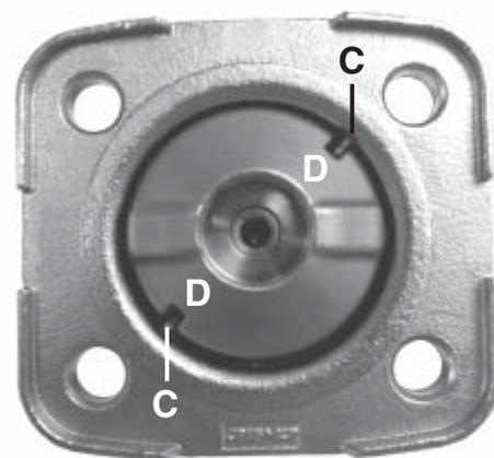
Place the compressor loosely on the actuator spindle, fit the grooves (D) into the guides (C). The compressor must be able to be moved freely between the guides!
