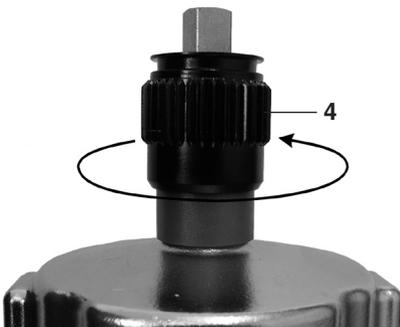
4. Unscrew the adjusting ring 4 and remove it.
