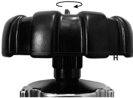
10. Push handwheel **H** in its original position on the square of the threaded spindle (observe the teeth of the adjusting ring 4 and the handwheel **H**). Tighten it with locking screw **6**.
