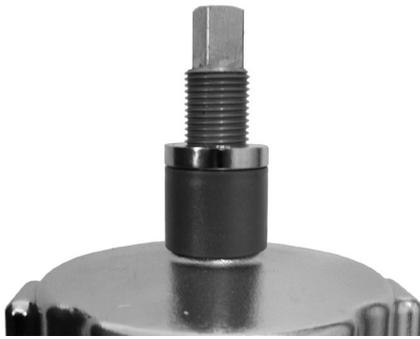
5. Dependent on the operating conditions, regrease the threaded spindle, especially a valve that is autoclaved. GEMÜ recommends grease Boss-Fluorine Y 108/00 (99099484)
